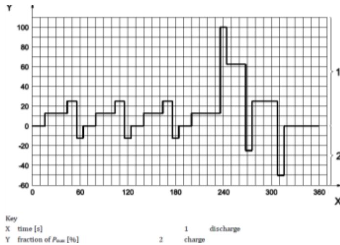
Figure 3: Profile for cycle life test – Dynamic discharge power profile A
