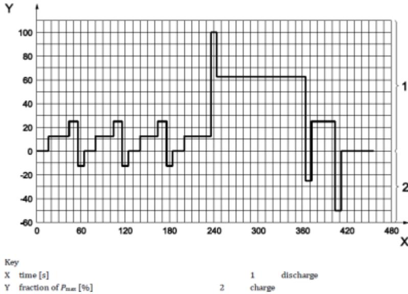
Figure 4: Profile for cycle life test – Dynamic discharge power
